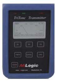
Simplex tone is applied to both the Tip to Ground and Ring to Ground simultaneously and can be heard even if one side of the pair is open.
