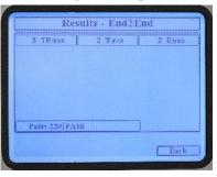
The left arrow, ◀, is pressed in the test viewer to display pair 229. This pair passed. The loop resistance indicates continuity from the Tip at the Local unit through the Remote unit back to the Ring at the local unit.
