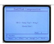
Select the appropriate desired pair and press **[F1] Start.** The **PR0** can be used for the compensation test. Connect the PR0 cords on each end and enter 0 for the pair on the E2E Comp screen.
