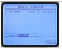
The measurements show a Tip to ground measurement of 2 ohms indicating Tip to Tip continuity.
