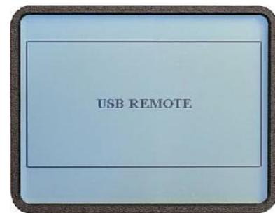
Disconnect the USB cable to exit the USB Remote mode. The ATV-25 will restart and return to the <Idle> screen.
