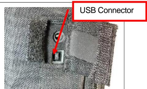
The ATV-25 automatically detects the USB connection and enters the USB Remote mode.
