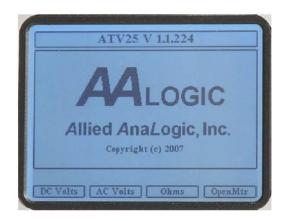
Connect a USB A-B cable from the PC to the ATV-25. A cable was provided with the ATV-25 for your convenience.
