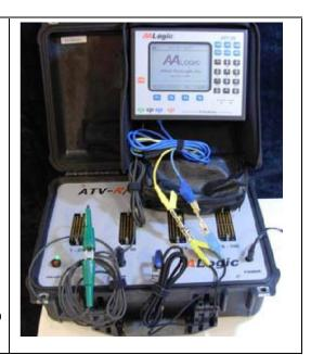
Press the [CFG] key on the ATV-25. The Configure main screen is displayed.
