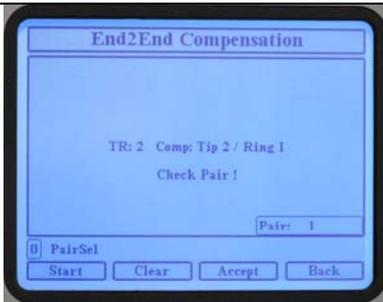
Select the appropriate desired pair and press **[F1] Start**. The **PR0** can be used for the compensation test. Connect the PR0 cords on each end and enter 0 for the pair on the E2E Comp screen.
