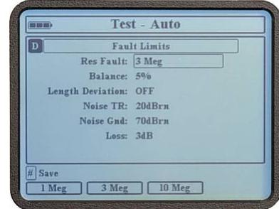
Verify the test information. The **Setup** should be completed for custom tests and the **Limits** set for the test.
