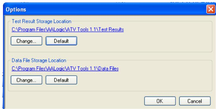
3. Click the **Change** button to change the path for either the Test Results or the Data Files. The paths are completely independent of one another.
