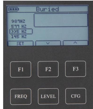
5. The ST-101 slowly increases the voltage level using the selected frequency until the last level used in buried mode is reached or the power limit is reached.
