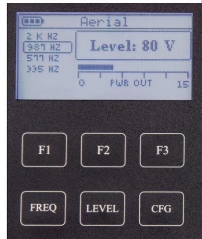
9. Output level is manually adjusted by pressing the **[LEVEL]** key. Use **[F2]** ↓ and **[F3]** ↑ to decrease or increase the voltage Level then press **[F1]** **SET**. The ST-101 returns to the transmit screen.
