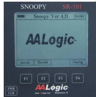
The SR-101 shows the Buried receive screen. The settings are the same as the last time the unit was used for Buried fault location. This is for convenience when starting and stopping location tasks on the same fault.
