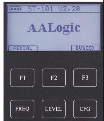
2. The ST-101 prompts to “**Connect Output**”. Connect the clips as described in 12.1.1 above and press **[F1] START**.
