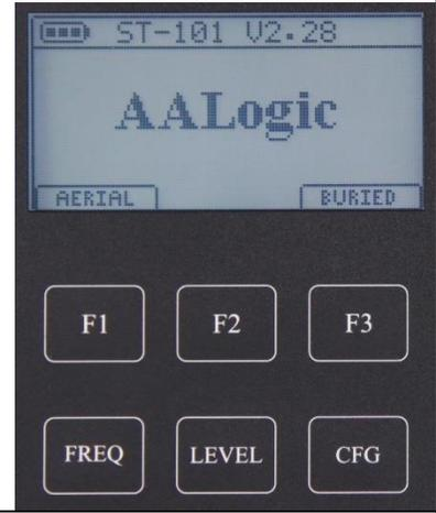
2. The ST-101 prompts to “**Connect Output**”. Connect the clips as described in 13.2 above and press [F1] **START**.
