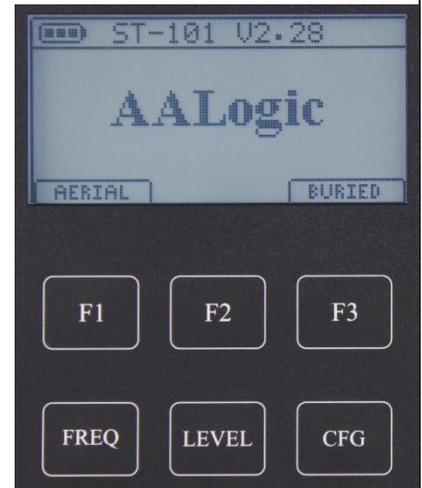
3. The ST-101 prompts to “**Connect Output**”. Connect the clips as described in 13.2 above and press [F1] **START**.
