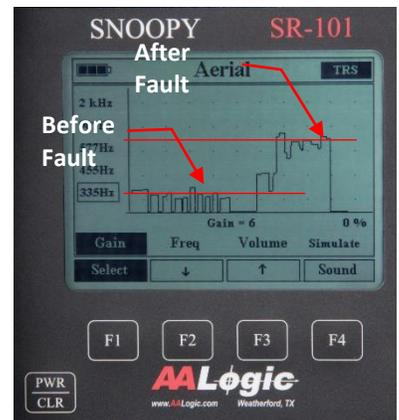
*Note: The cable pair and group are twisted inside the cable. This means the pair may be on the top, bottom, or middle as the probe is moved along the cable. It is normal for the signal indication to rise and fall while monitoring the cable. The fault location is determined by higher average signal peaks before the fault than after the fault for shorts and crosses. The average peaks are higher after a split.*
