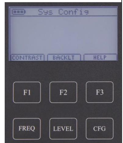
2. Press [F1] **CONTRAST** or [F2] **BACKLT** to select the setting to adjust. Use the [F2] **↓** and [F3] **↑** to adjust the setting and press [F1] **SET** to save and exit the [CFG] mode.
