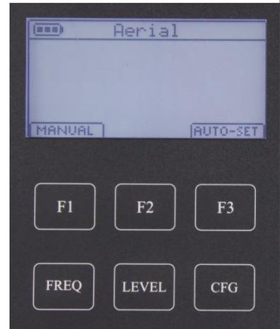
The [F3] **AUTO-SET** mode is the easiest way to start unless you want to use the last frequency or set a specific frequency. You can adjust the frequency and/or the level after the ST-101 begins transmitting.
