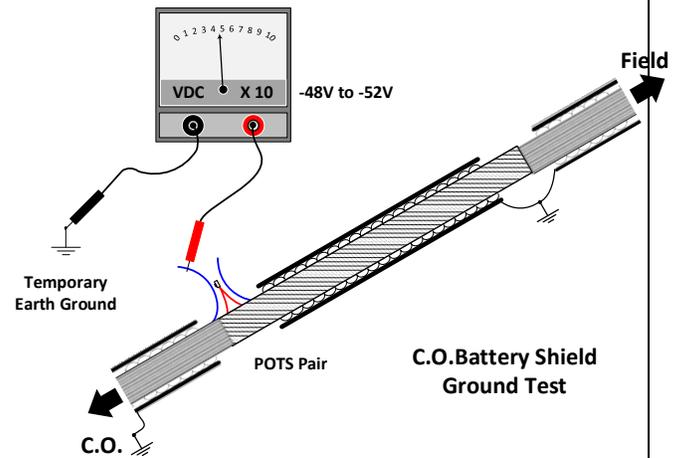
7. Connect a strap between the ring and the shield toward the C.O. The voltage reading should drop to less than -1V if the shield is good and there is a good ground.
