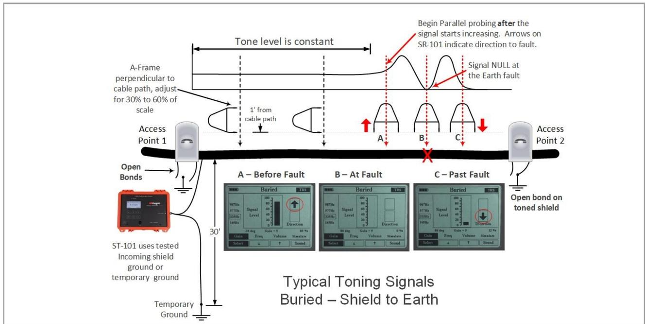
Typical Toning Signals Buried – Shield to Earth
