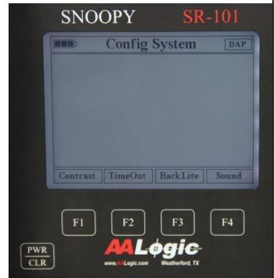
This timeout can be set in 15-minute increments from OFF to 45 minutes. As shown, the SR-101 remains on until the user turns it off with the [PWR/CLR] or the battery is exhausted.
