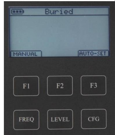
The **AUTO-SET** mode is the easiest way to start unless you want to change the frequency. You can adjust the frequency and/or the level after the ST-101 begins transmitting.
