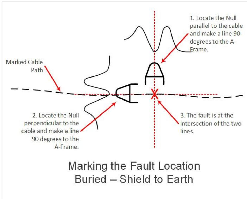
Marking the Fault Location Buried – Shield to Earth
