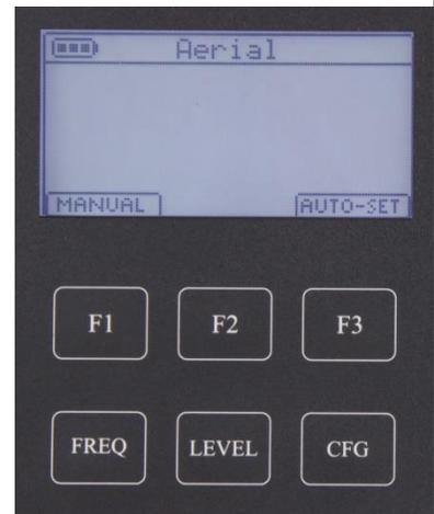
4. The ST-101 prompts to select a frequency. Use **[F2] ↓** or **[F3] ↑** to highlight the desired frequency then press **[F1] SET**. The frequency last used in aerial mode is pre-selected. The screen includes a suggested section length for each frequency.
