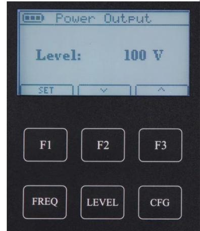
9. The frequency is manually adjusted by pressing the [FREQ] key. Use [F2] ↓ or [F3] ↑ to highlight the frequency then press [F1] **SET**. The ST-101 returns to the transmit screen.
