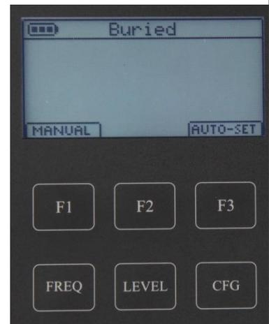
4. The last used frequency in buried mode is automatically selected in the list on the left. Use [F2] ↓ or [F3] ↑ to highlight the desired frequency then press [F1] **SET**. The ST-101 returns to the transmit screen.
