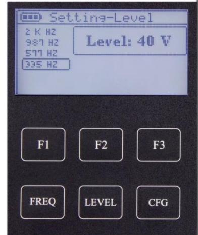
6. The ST-101 starts transmitting the signal at the frequency and level determined by the scan. Follow the instructions for the receiver to ensure the signal is detected by monitoring the cable.
