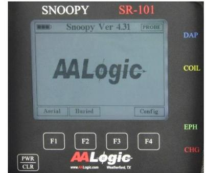
The SR-101 shows the Aerial receive screen. The settings are the same as the last time the unit was used for Aerial fault location. This is for convenience when starting and stopping locating tasks on the same fault.
