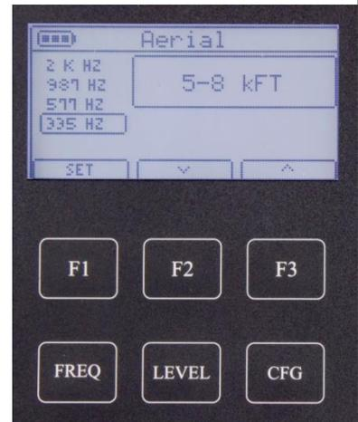
5. The ST-101 uses the selected frequency and gradually increases the voltage to obtain an initial Level. This level should be sufficient in most cases. The frequency and gain on the receiver must also be adjusted on the SR-101.
