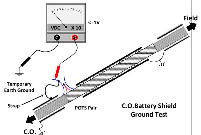
10. Repeat the test for the field side shield at the access point.
