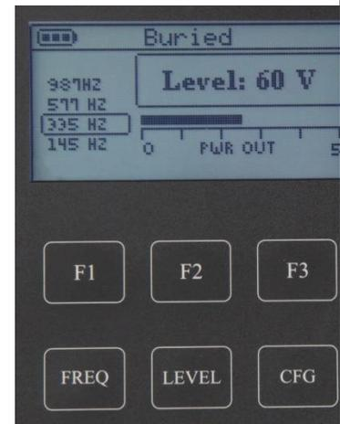
8. Voltage level is manually adjusted by pressing the [LEVEL] key. Use [F2] ↓ and [F3] ↑ to decrease or increase the voltage Level then press [F1] **SET**. The ST-101 returns to the transmit screen.
