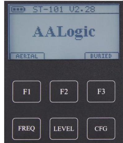
3. The ST-101 prompts to “**Connect Output**”. Connect the clips as described in 12.1.1 above and press [F1] **START**.
