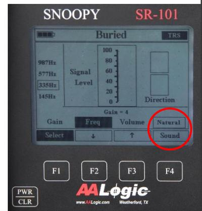
5. Insert the A-frame in the Earth approximately 1' from the previously marked cable path, refer to 13.6 below. Adjust the **Gain** to obtain a graph signal that peaks between 30% and 60%. The graph in the center shows the signal level. There is also a percentage shown below and right of the arrows.
