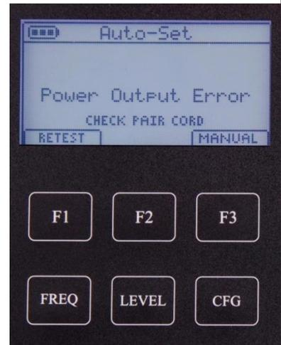
7. The ST-101 starts transmitting. Follow the SR-101 instructions below to ensure the signal is detected by monitoring the cable approximately 10 feet from the connection point.
