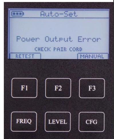
7. **Set SR-101 to XXX Hz.** In the example, ST-101 has successfully determined a starting frequency of 987. Set the frequency on the SR-101 receiver. Press **[F1]** **OK** to continue and start sending tone.
